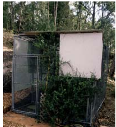
Outside aviary (purpose built) Recommended size 2400mm high by 2400 wide by 4800 deep
